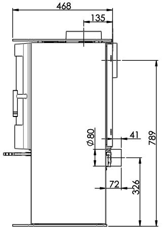
The direct air intake spigot (80mm diameter) to the rear of the stove is removable with a 2.5mm Allen key.
