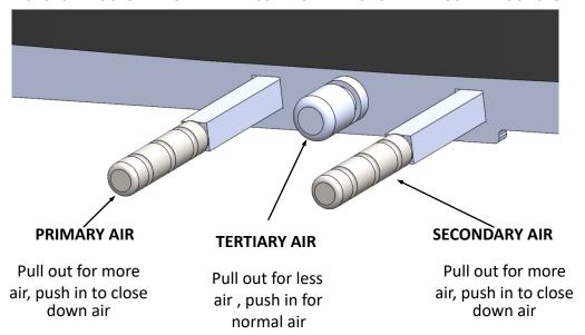
Air regulation; The three control levers perform differing tasks in regulating the combustion air on your appliance:
