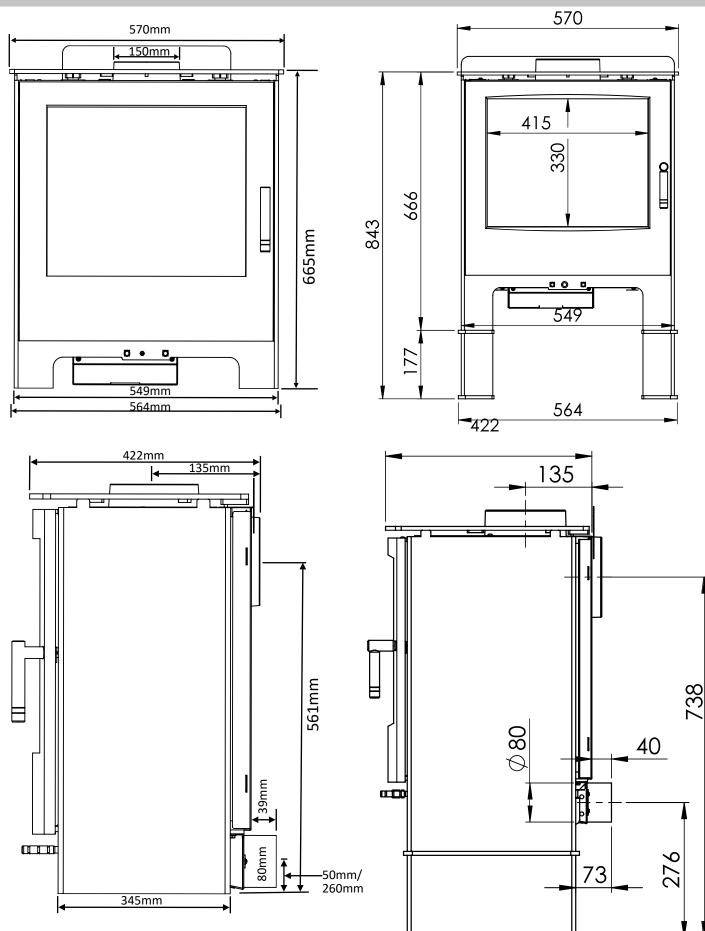
The **direct air intake spigot** (80mm diameter) to the rear of the stove is removable with a 2.5mm Allen key.
