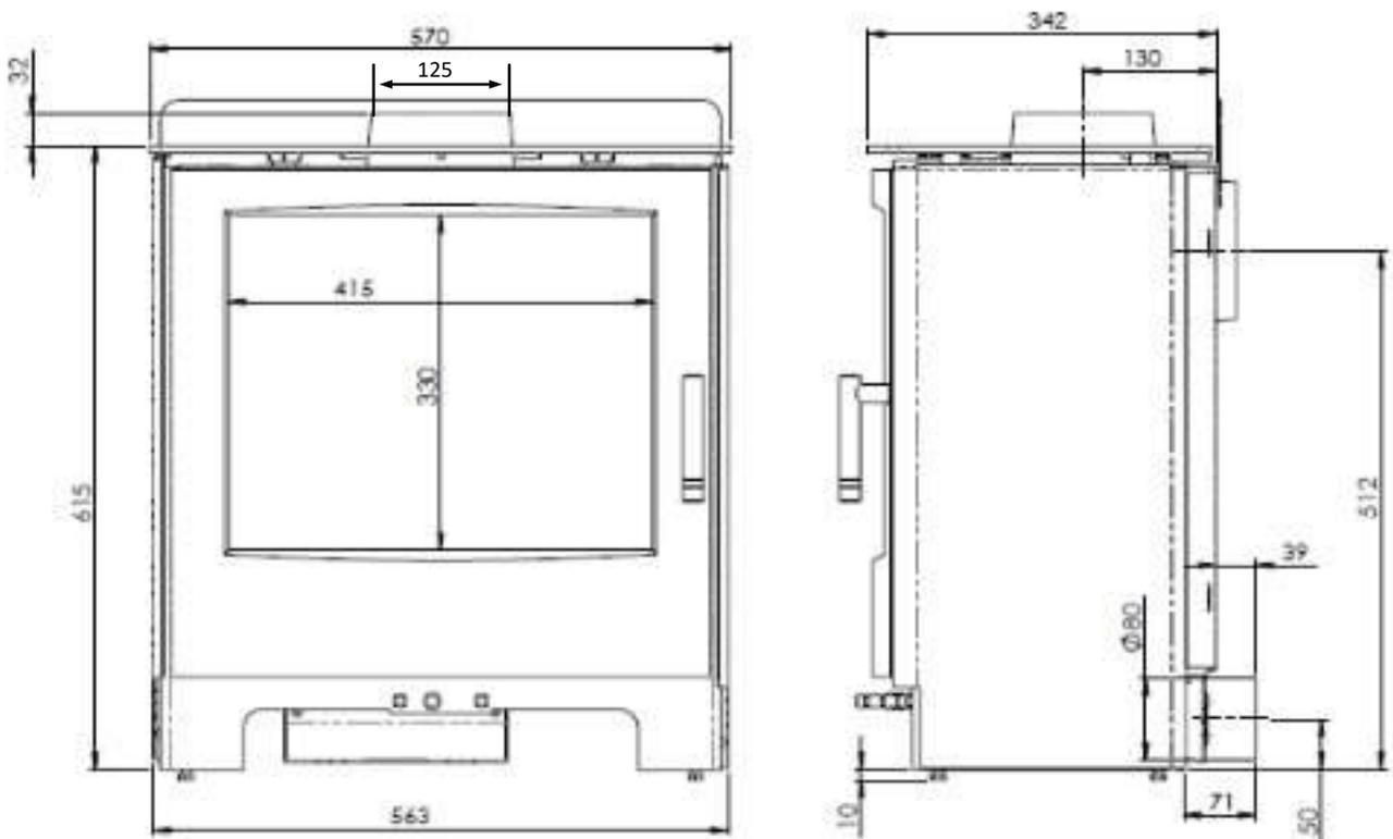
The **direct air intake spigot** (80mm diameter) to the rear of the stove is removable with a 2.5mm Allen key.
