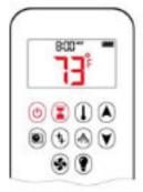
To change between °C and °F, press ® and I buttons simultaneously.
