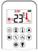
If Thermostatic, Program or Eco Mode is activated, the corresponding icon and "RPP" is displayed on the handset.
